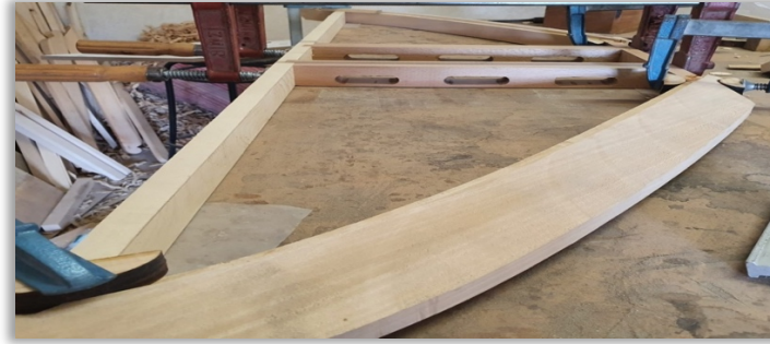
Photo 4. Skeleton form of the Unified Kanun during the construction stage
