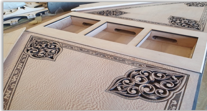
Photo 8. Final state of the middle section of the Unified Kanun before drilling the pegs
