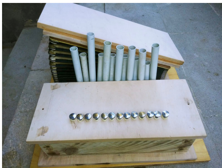
Photo 2. Prototype of the Azerbaijani Ergän developed by Enver Sadıkov and Teymur Hüseynov at the Azerbaijan National Conservatory on the basis of Abd al-Qadir al-Maraghi's descriptions and historical organological sources (Author's personal archive).
