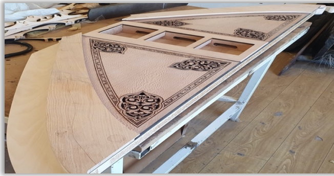
Photo 7. Unified Kanun with the top boards attached and the tuning peg boards glued
